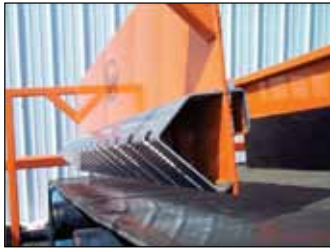
Stitch weld hanger to hopper (45° shown)
